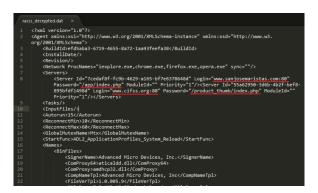
The XML config file shows the C&C proxy server addresses. According to the information in <Servers> section, two URLs are used to establish the connection with the C&C proxy, which is merely a someone's hacked website.
